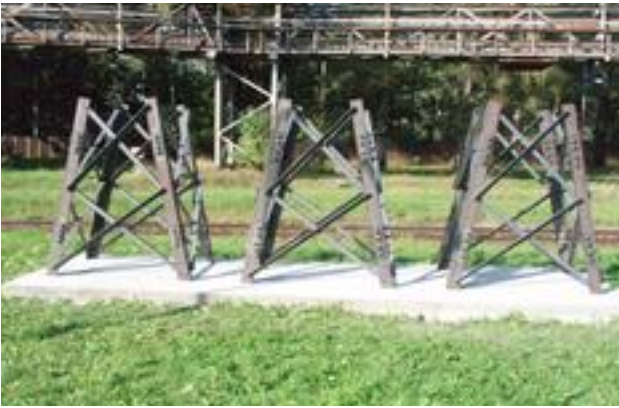
Atmospheric corrosion resistance testing polygon.
